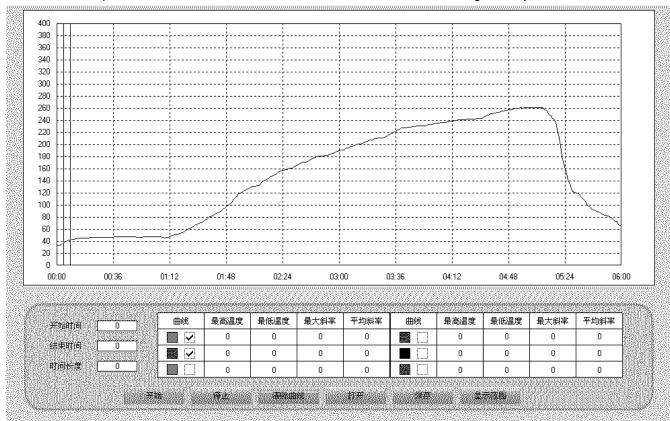
Figure 1 – Solder Reflow Profile Tested
