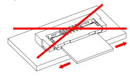
3) Due to the structure of the connectors, they do not have string resistance to upward pulling; therefore, support the FPC/FFC when a pulling force is applied to it.
