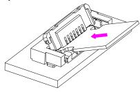
3) Rotate down the actuator until firmly closed. It is critical that the inserted FPC/FFC is not moved and remains fully inserted. Should the FPC/FFC be moved, open the actuator and repeat the process, starting with Step 1 above.
