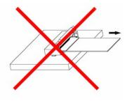
Do not add the load mating FPC/FFC with connector housing.
