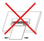
Due to the structure of the connectors, they do not have string resistance to upward pulling; therefore, support the FPC/FFC when a pulling force is applied to it.
