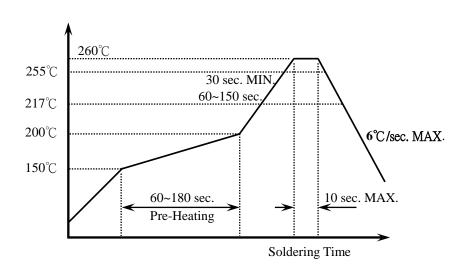
Figure 1. Recommended Reflow Temperature Profile
