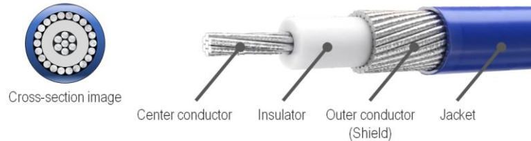
Coaxial cable structure
